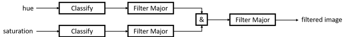
Figure 15: Signal flow diagram of Filter Chain
